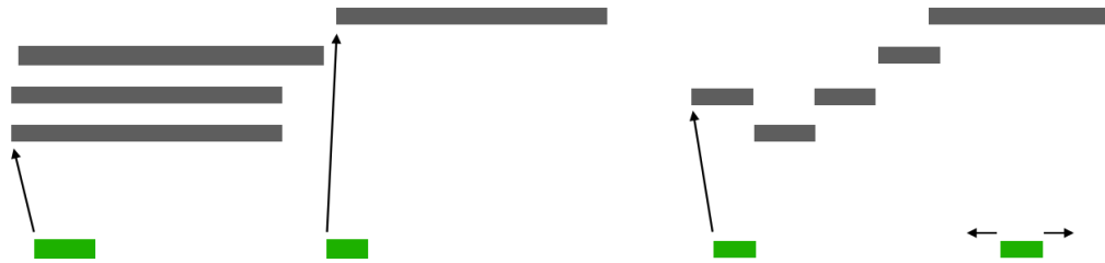
Figure 4: Illustration of the marker alignment helper function. Notes are presented in a piano roll fashion where grey notes belong to the original track and green notes are the beat or phrase markers from the other track.
